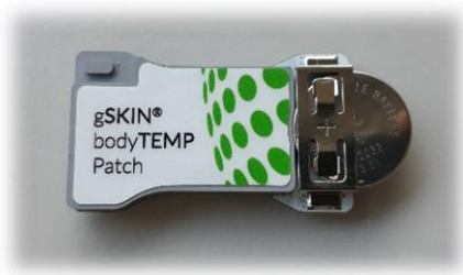
Figure 1 – The logging device: gSKIN® BodyTemp patch
