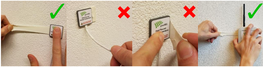
Figure 4: How to remove the nodes/sensors correctly (left) and incorrectly (right)
