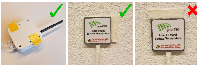
Figure 3: How to mount the node correctly (left), the sensor correctly (middle) and incorrectly (right).
